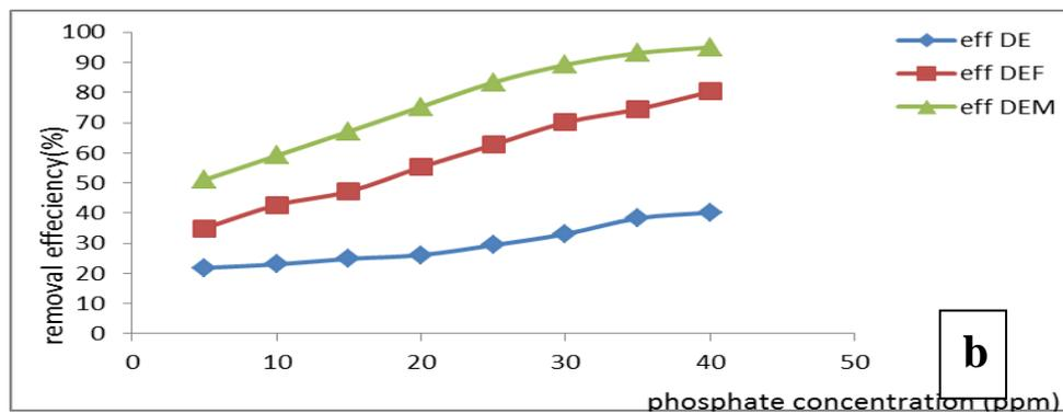
Figure 4: The efficiency of removal phosphate ions by DE, DFe and DED at different concentrations
