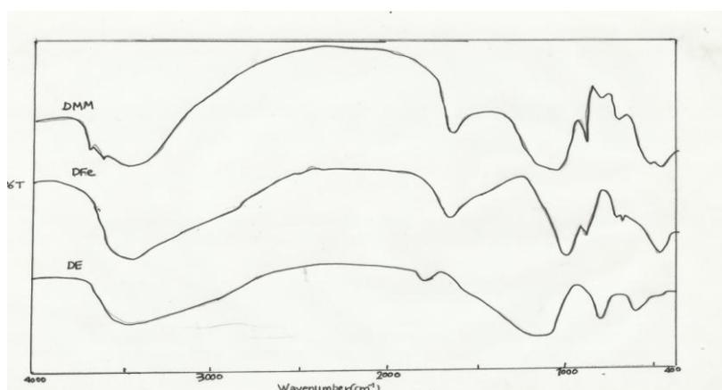
Figure 1: IR. Spectrum of diatomite and modified diatomite
